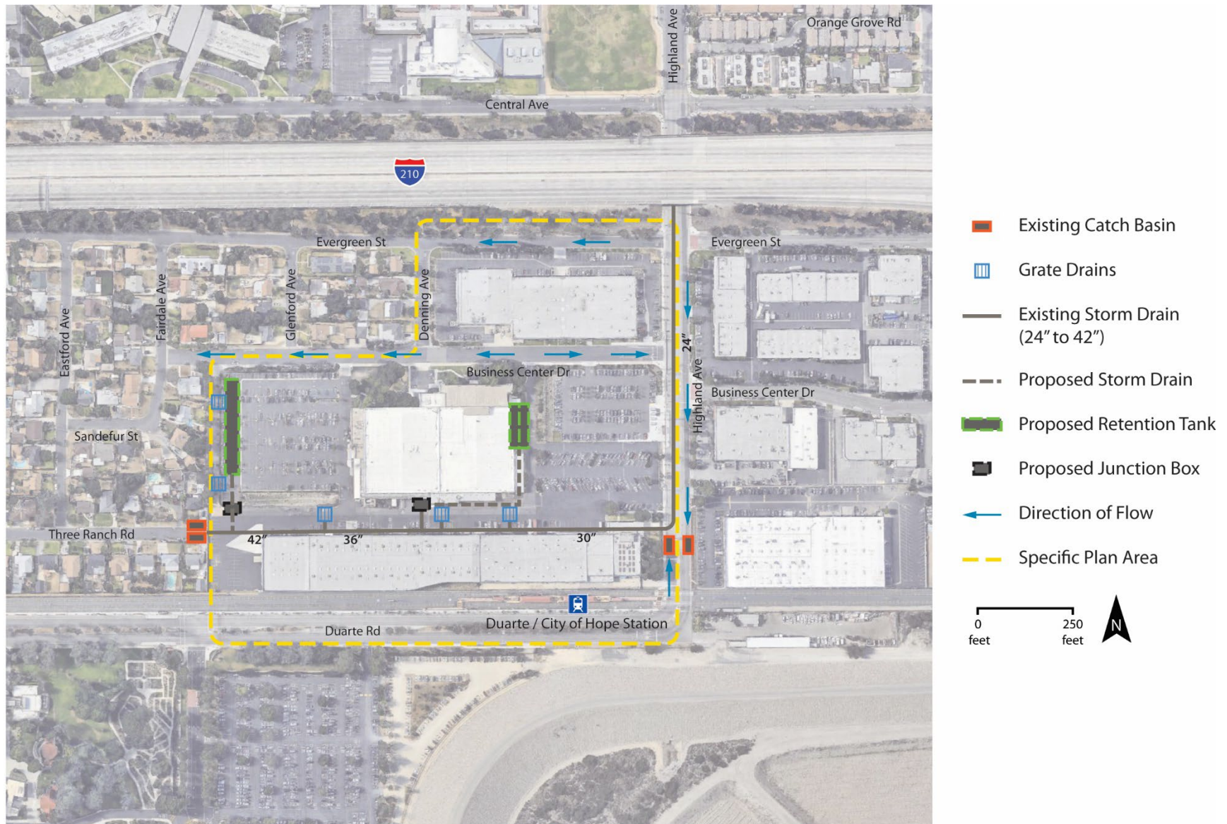
Figure 4-4: Stormwater Infrastructure Plan
